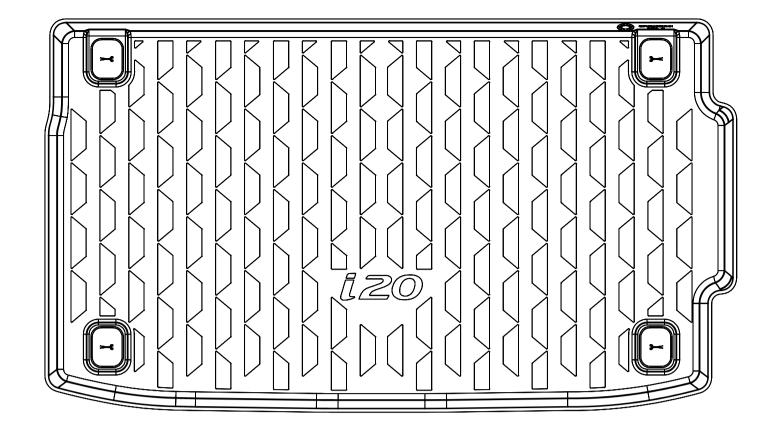
Q0122ADE10 - Trunk liner (for vehicle with luggage board and without subwoofer in trunk area)
